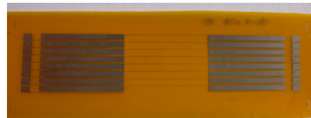
Figure 9: New HFS with thin film technology (wire thickness 30 \mu m) [28]
