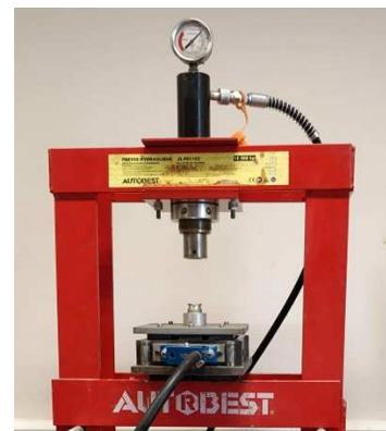
Figure 2 : a. Samples of concrete molded for mechanical tests in stainless steel molds with a vibration system, b. Samples in the mold on the hydraulic press.
