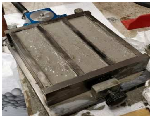
Figure 2 : a. Samples of concrete molded for mechanical tests in stainless steel molds with a vibration system, b. Samples in the mold on the hydraulic press.
