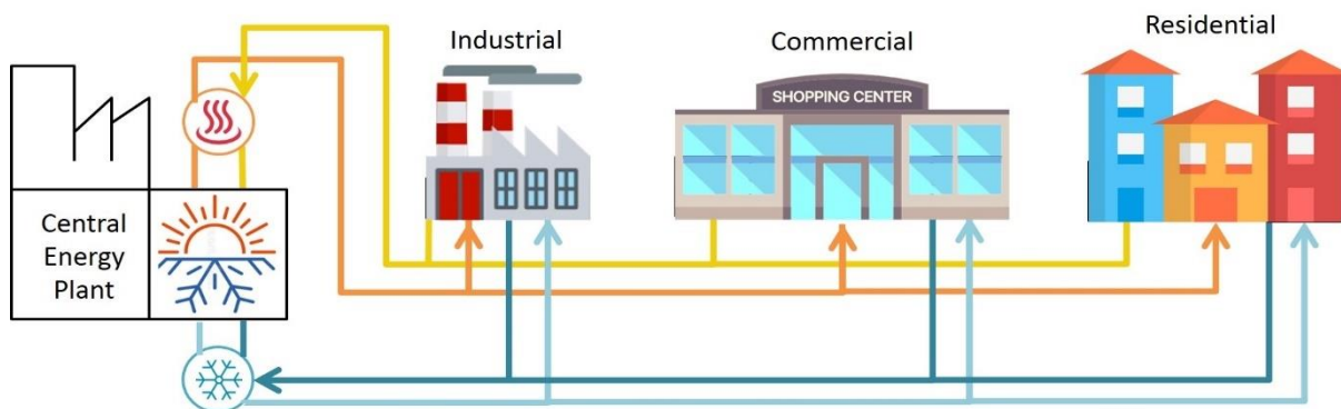
Figure 1. General scheme for a DHC system
