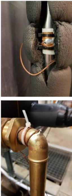
Figure 4: Thermocouples immersion sleeves: surface and elbow thermocouples
