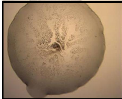
Emulsion moving towards the center t_0 + 7.5 \text{ min} , T = 8^\circ\text{C}
