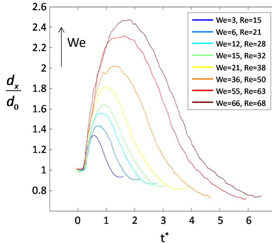
*Time evolution of the horizontal spreading for drops made of 40% water and 60% glycerol by volume.*
