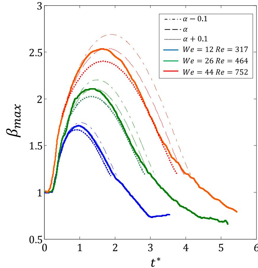
*Illustration of the sensitivity to the adjustment of  $\alpha$ .
