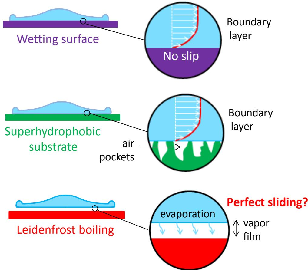
*Mechanisms for the frictions at the bottom edge of the droplet*
