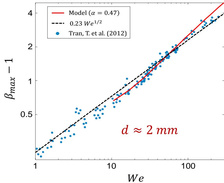
Verification of the independence of  $\beta_{max}$  on the droplet size
