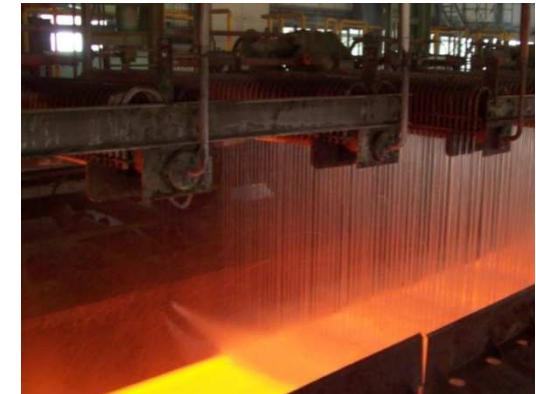
*Cooling of a steel band by water sprays
