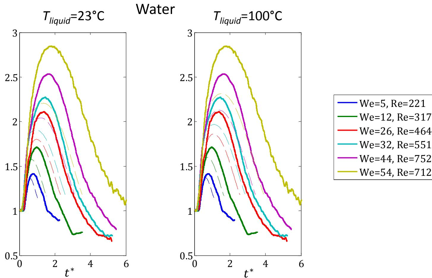
*Influence of the temperature used to calculate the liquid properties ( $\rho, \mu, \sigma$ )*
