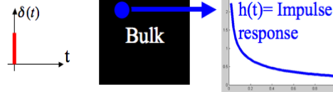
Figure 8. Impulse response of the bulk.
